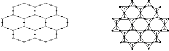
Fig. 2(a) Fig. 2(b) Fig. 2. Construction of silicate network SL(n) from HC(n)
