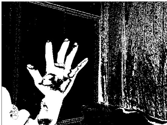
Fig. 3. Image HAND_1 . The hand and arm are set to white, denoting foreground. Curtains are also set to white as it is moving due to the breeze.
