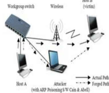
Fig. 1. Implementation of ARP poisoning
