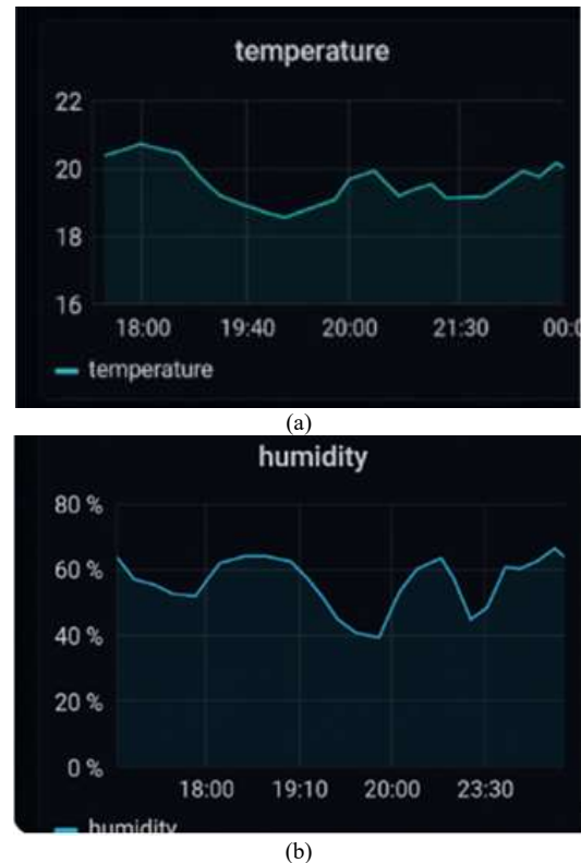
Fig. 6. Grafana dashboard with 2 time-series. (a) Temperature. (b) Humidity. Note: RH and air temperature are digital channels (no host ADC); soil moisture is analog (ADC-based).
