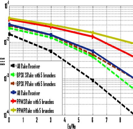
Fig. 4. Performance of PPM and BPSK modulations.
