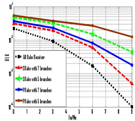
Fig. 6. BPSK performance for different rake receivers.
