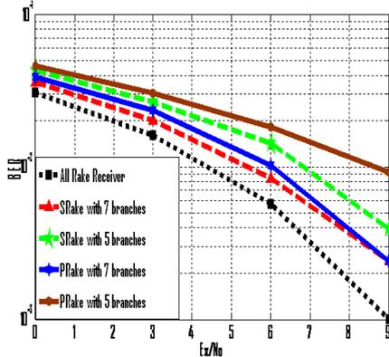
Fig. 2. PPM performance for different rake receivers.
