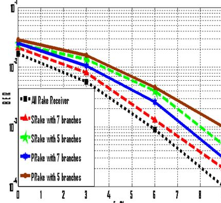
Fig. 3. BPSK performance for different rake receivers.
