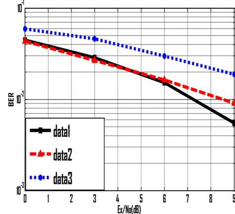
Fig. 7. Performance of all-rake, s-rake and p-rake.
