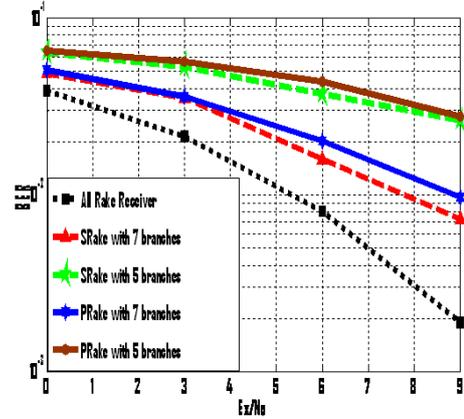
Fig. 5. PPM performance for different rake receivers.
