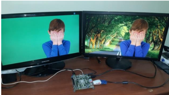
Fig. 10. FPGA-based real-time evaluation of the designed Chroma-key effect system.
