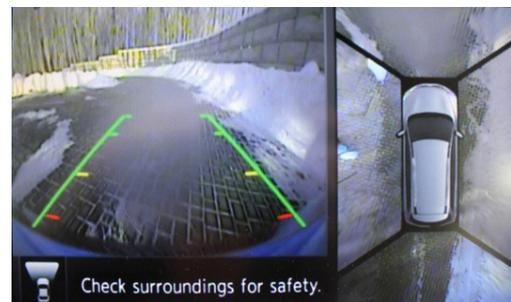
Fig. 1. Nissan Around view monitor system.
