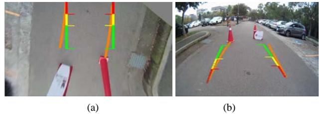
Fig. 9. The parking guiding lines. (a) drawn on the top-view image. (b) drawn on the original image.
